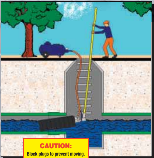
A model #705 E-Z Plug Adaptor shown with the new 8" SST Plug
